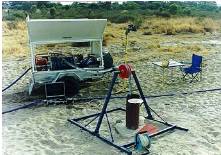
Test pumping equipment
