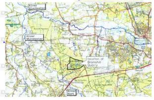
A desktop study was conducted to determine the suitability of a quarry for development as a landfill site, via 'disperse & attenuate' or containment, and the availability of on-site development materials. Data on the geology, hydrogeology, meteorology, geography & current site operations was collated and reviewed and a walk over survey was conducted.
